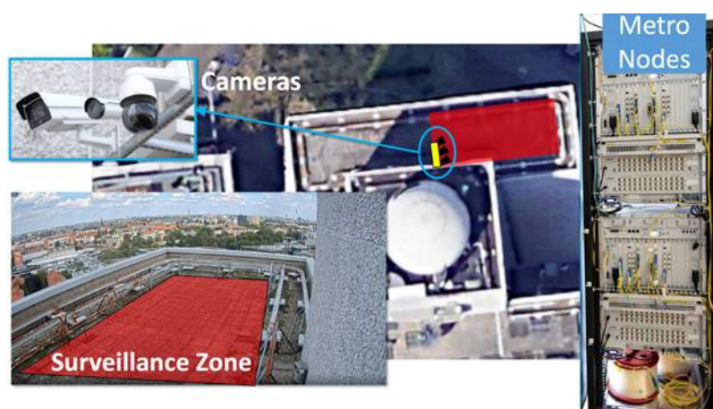
Figure 2: Deployment of the demonstrator: (left) Surveillance zone on the rooftop of the Fraunhofer HHI building in Berlin. (right) Installed surveillance cameras and deployed optical metro network equipment
