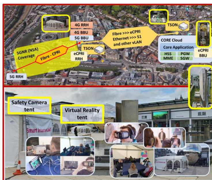
Figure 2: Smart City trial deployment in the city of Bristol, UK
