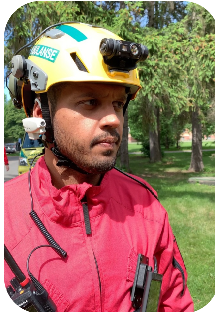
Figure 7 USAR suit with BlueEye camera installed (photo: Andreas Gustavsen)
