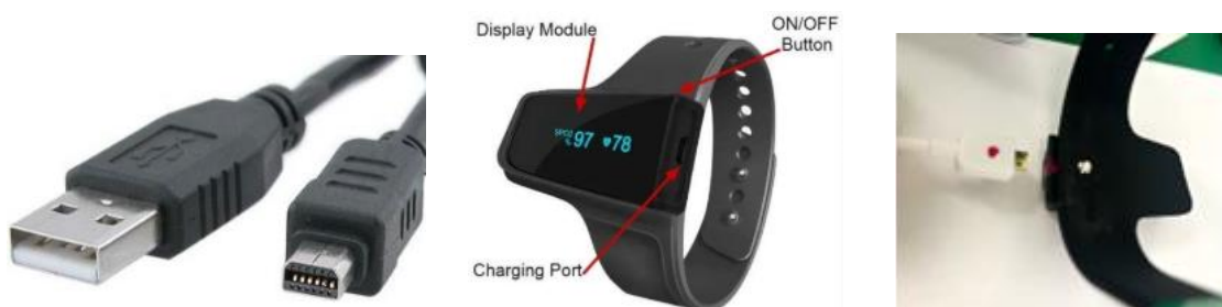
Figure 3 Micro-D charging cable (L); SpO2 sensor watch (M); Red dot marked on SpO2 charging cable and watch (R)
