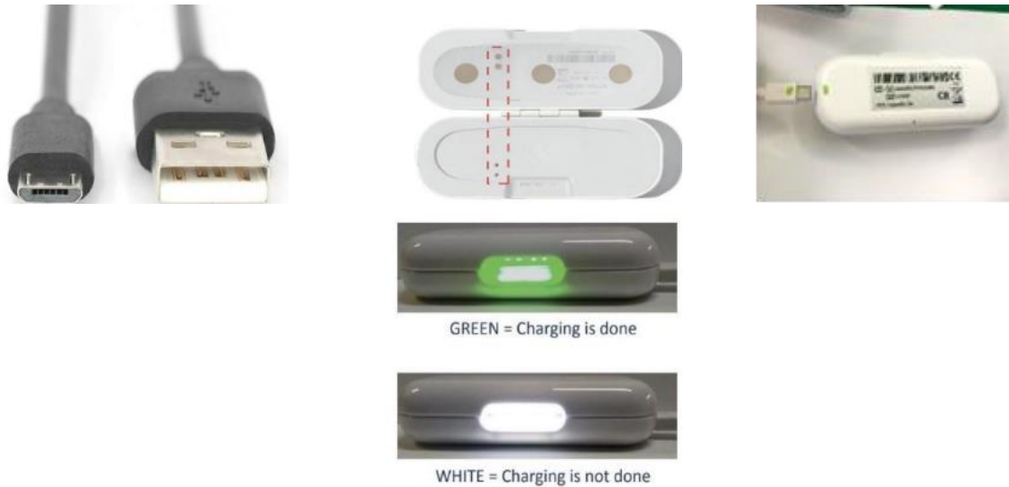
Figure 2 Micro-B charging cable (L); two charging dots in MVS case (M); Green dot marked on MVS patch and charging cable (R)
